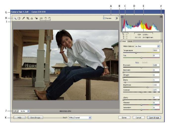
Camera Raw dialog box A. View options B. Click the Basic or Detail tab to access different controls C. RGB values D. Histogram E. Image settings F. More menu G. Camera and some EXIF information H. Tools I. Rotate buttons J. Zoom levels K. Bit depth options
