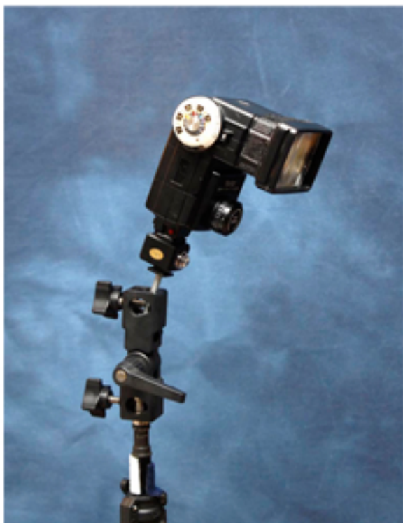
$80 flash unit with light stand and bracket used as hair light
